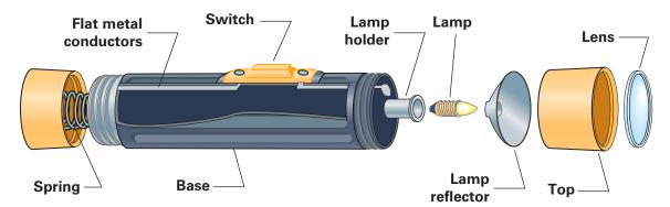
Fitting Together A flashlight has parts made from different materials. All the parts have to fit well and work together. What parts of a flashlight are purchased from other companies?
